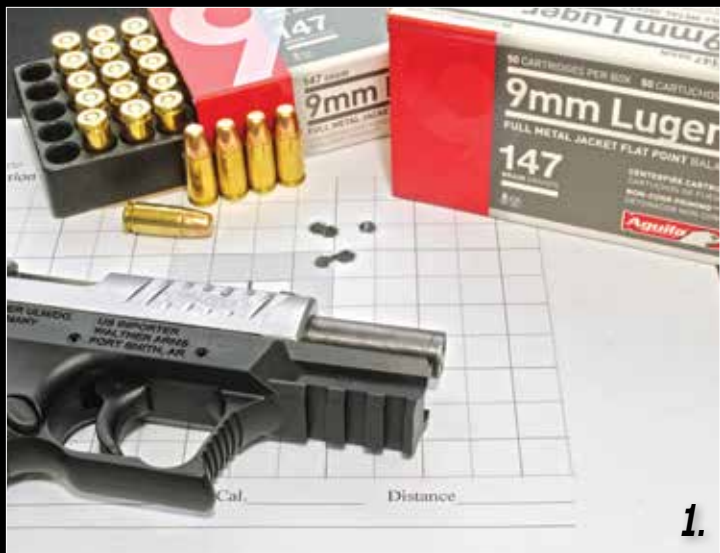
1—AGUILA'S 147-GR. FLAT POINT TRAINING AMMO WAS THE MOST ACCURATE LOAD OF THE DAY IN OUR CCP M2 TEST PISTOL. THIS SUB 1-INCH GROUP WAS FIRED AT 15 YARDS WITH NOTHING MORE THAN A RANGE BAG SUPPORTING THE AUTHOR'S WRISTS. RECOIL WAS STILL VERY MANAGEABLE LARGELY DUE TO THE SOFTCOIL TECHNOLOGY.
