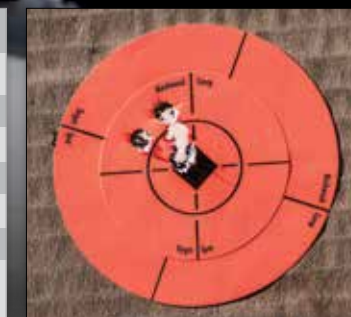
GROUPS TESTED USING A BAG FOR A REST ON THE HOOD OF A TRUCK. BEST GROUP SHOWN OUT OF FIVE 5-SHOT GROUPS FROM 100 YARDS. VELOCITY MEASURED USING A CHRONY CHRONOGRAPH.
