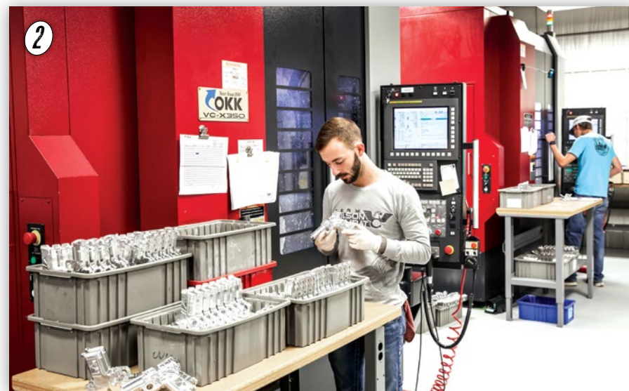
1 —FIREARM COATING? YOU GOT IT — ALSO DONE IN-HOUSE. 2 —A BATCH OF WILSON COMBAT'S OUTSTANDING EDCX9 DOUBLE-STACK PISTOL FRAMES BEING INSPECTED PARTWAY THROUGH THE MACHINING PROCESS. 3 —TEST FIRING FOR FUNCTION AND ACCURACY IS DONE BY HAND — A PROCESS EVERY FIREARM GOES THROUGH BEFORE IT LEAVES THE WILSON COMBAT FACTORY.
